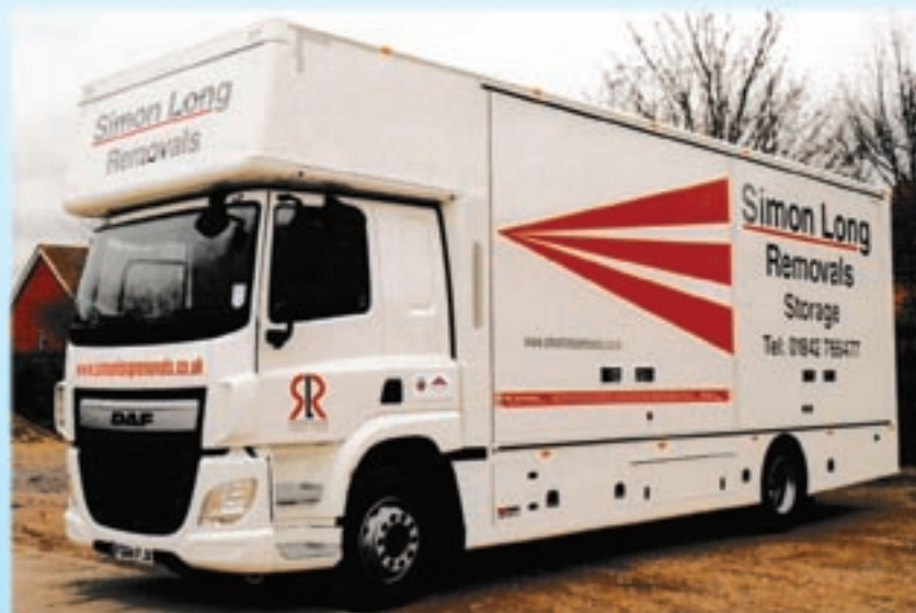
New DAF CF chassis with sleeper cab and four container luton body.
