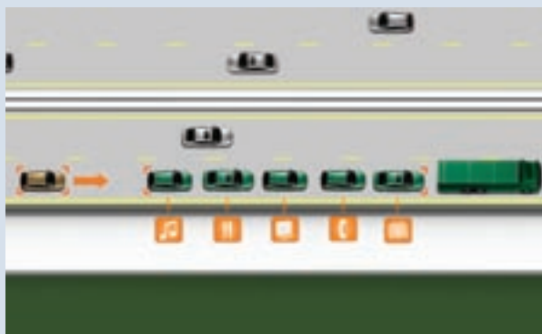
● SARTRE technology makes it possible for multiple vehicles in a road train to integrate smoothly with other traffic on public motorways.
