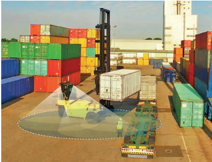
● Hyster's object sensing system uses multiple sensors.
